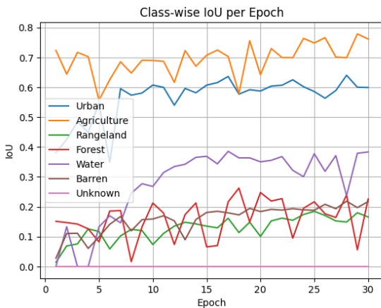
Figure 8. Per-class IoU of validation set across training epochs when using ResNet encoder
