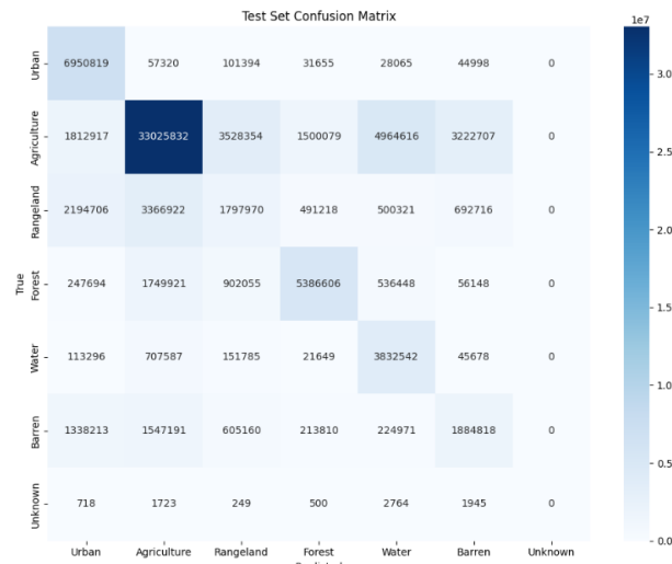
Figure 5. Confusion Matrix at Test Time(Focal loss). Compared to baseline, the amount of Agricultural land being incorrectly classified as Water increased.
